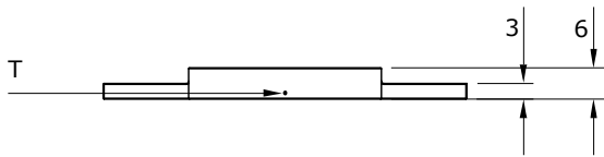
Figure 4 IHF01 dimensions in \times 10^{-3} m. T marks the location of the thermocouple.
